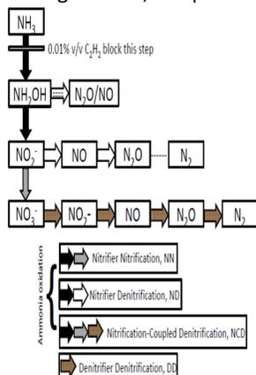
Fig. 1 the main pathways of N<sub>2</sub>O production in soil
