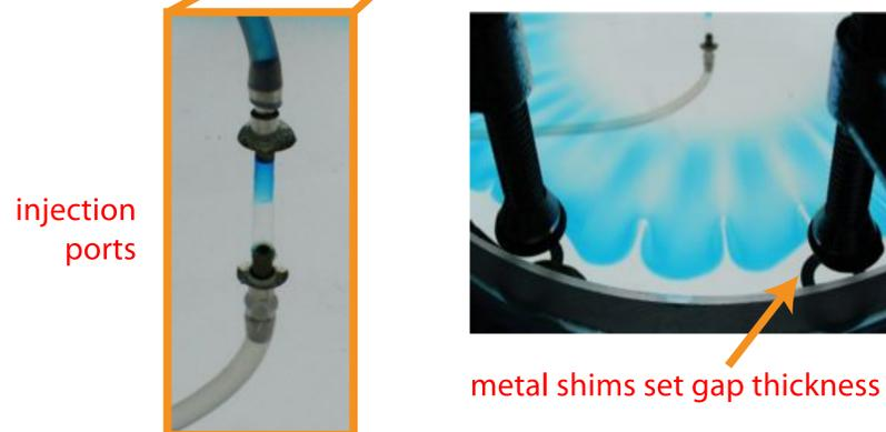
This setup allows for the systematic variation of three control parameters: injection rate, viscosity ratio, and gap thickness.
