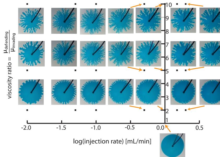
We observe that fingering occurs for all viscosity ratios larger than one, and that the size of the compact core depends largely on the viscosity ratio.
